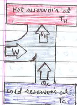
fig (a) Energy flow dia. of a practical refrigerator
